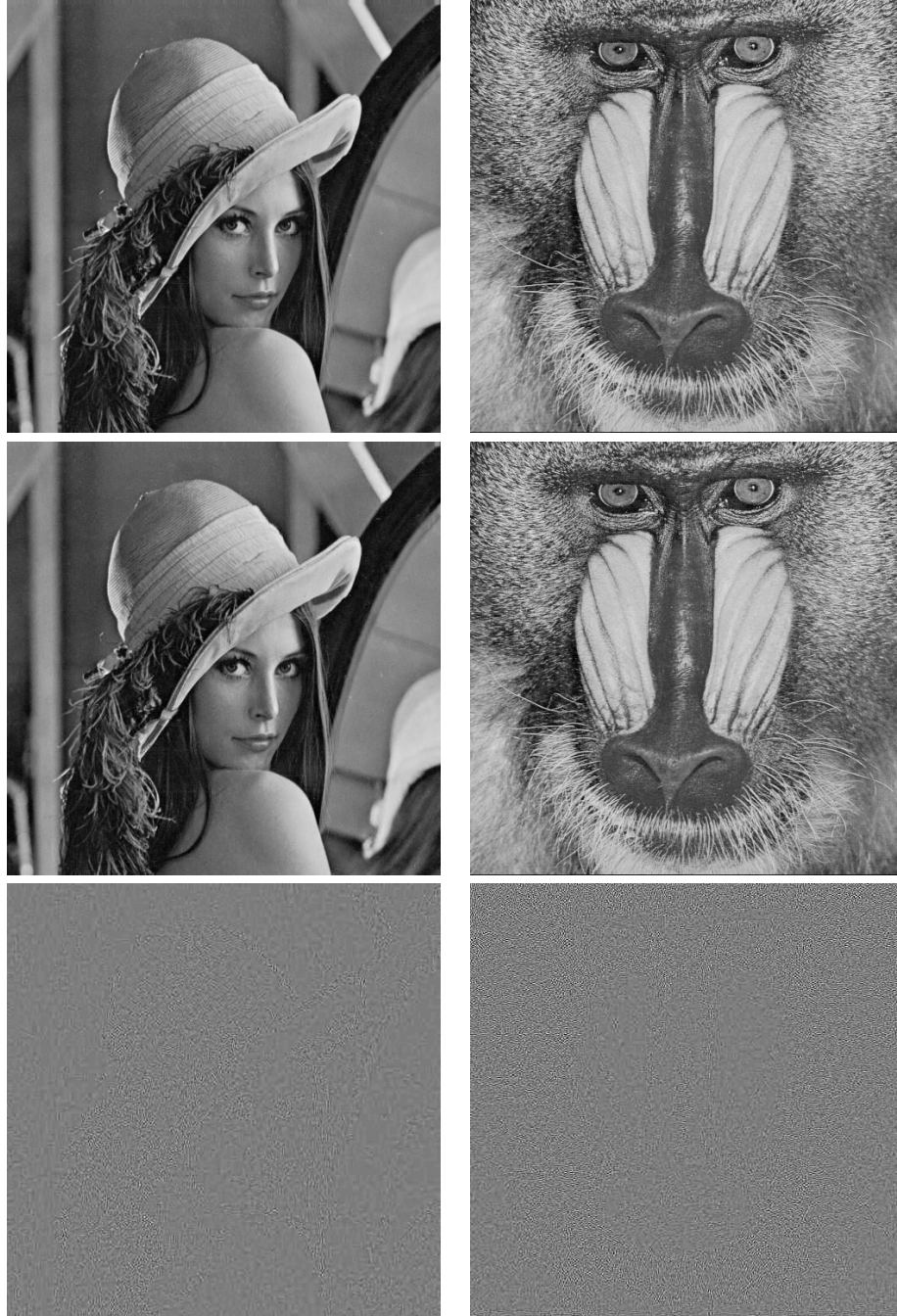
Figure 6: The original images (top), fingerprinted images (middle), and difference images (bottom) for Lenna and Baboon. In the difference images, gray color indicates zero difference between the original and the fingerprinted version, and brighter and darker indicates larger difference.
